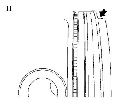
If the described failure is detected the usage of correct fuel has to be verified. A fuel and engine oil sample has to be analysed for diesel contamination. Furthermore the fuel filler neck has to be checked for any damages (the useage of a diesel nozzle widens the diameter of the fuel
